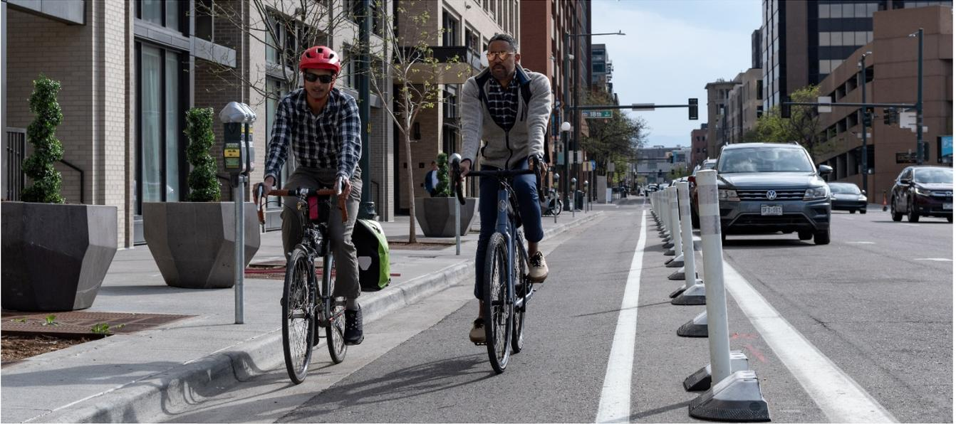
Image 15: Separated Bike Lane with Flex Posts in Denver, CO
