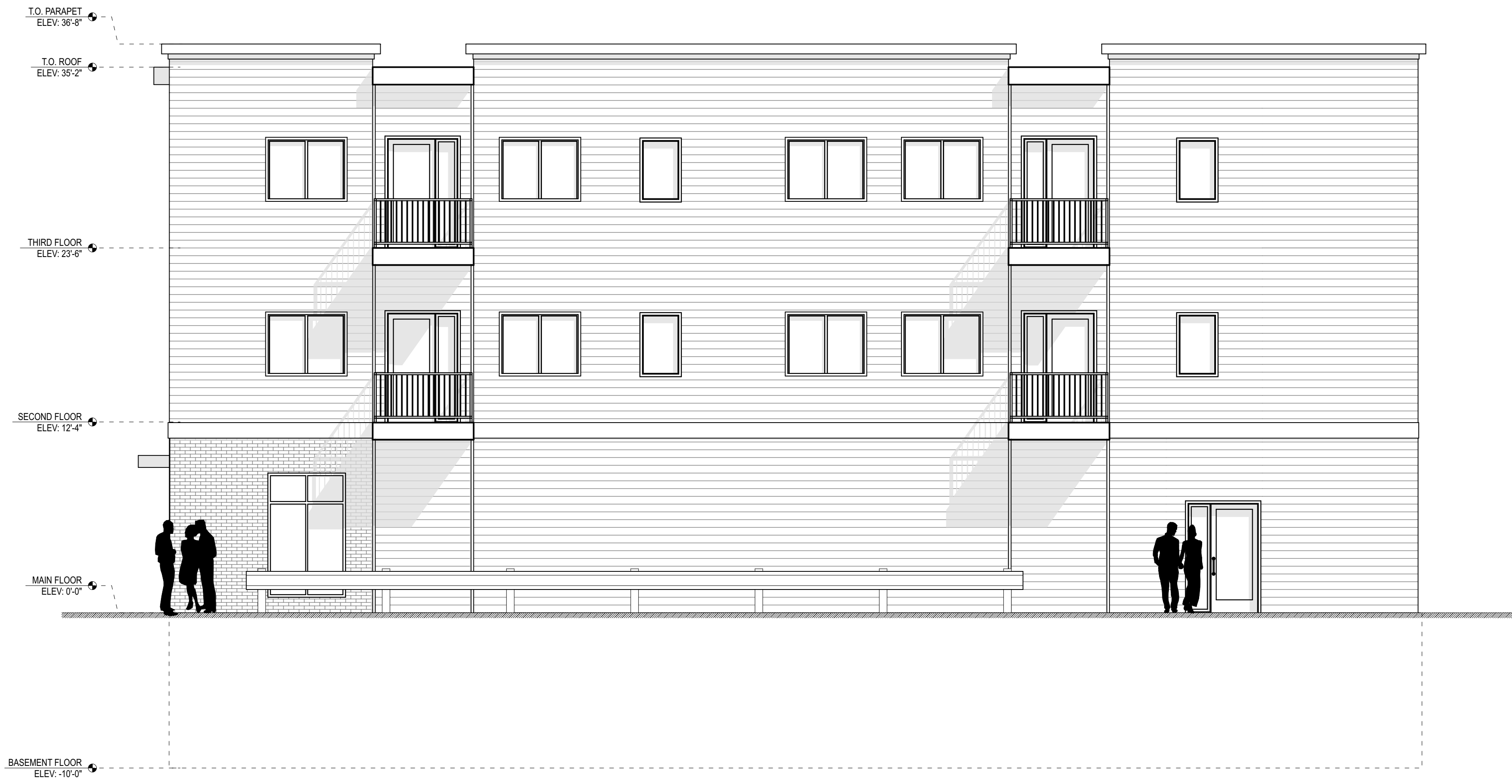
2 WEST ELEVATION SCALE: 3/16" = 1'-0"
