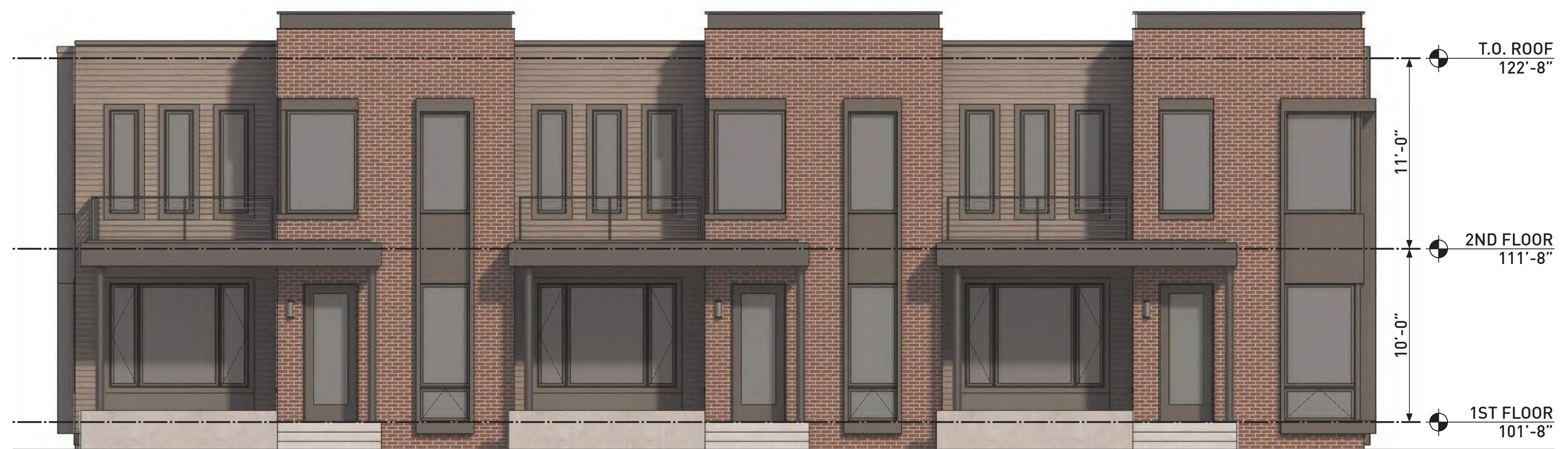
BUILDING A - FRONT ELEVATION (B,C,D,E,L & M SIMILAR)
