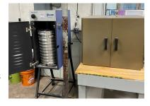
For aggregate testing, we have a 7.0 cubic foot drying oven, double burner hot plate, floor model sample splitter, a Gilson Silent Sifter sieve shaker, tabletop aggregate washer and a AND GP-100KS precision balance. Our equipment allows Benesch to be able to handle a large volume of samples in a short amount of time as necessary due to our large capacity oven and hot plate combination, allowing us to process up to 14 samples at one time.
